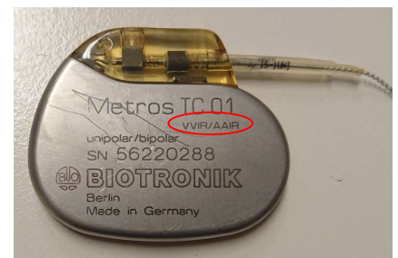
Figure 6. Sample device shown with the printed codes. This particular device can operate in two different
