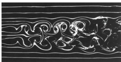
Fig. 3. Laminar and turbulent flow. Right next to the tube walls (at low speeds) the flow is laminar, but in the center (at high speeds) it is turbulent.
